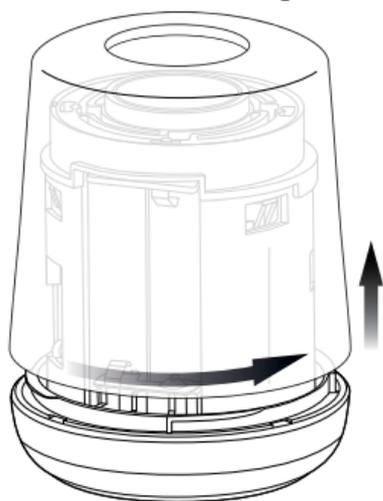
2. Insert the batteries correctly and press firmly to click into position.
