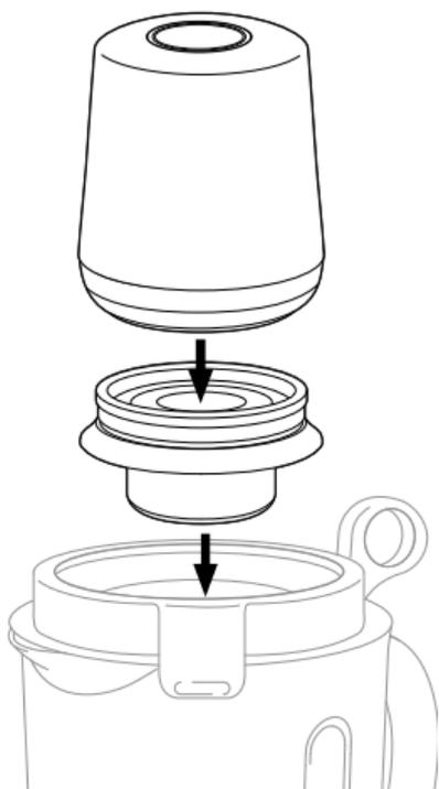
4. Press the POWER Button to turn on the Vacuum Pump. The Vacuum Pump will automatically stop once a vacuum pressure is reached.
