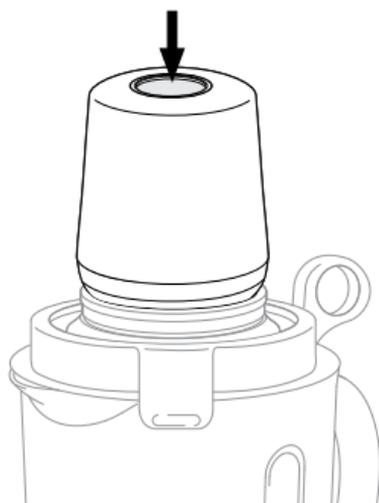
5. Remove the Vacuum Pump from the blender lid.
