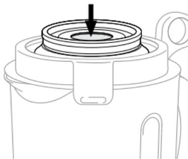
The Inner Cap with Vacuum Valve can now be left in the blender lid for any blending tasks, whether it be Vacuum-Blending or Non-Vacuum Blending.
