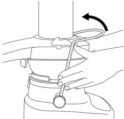
5. The safety locking arm should now be in a vertical position and locked into place on top of the juicer cover.
