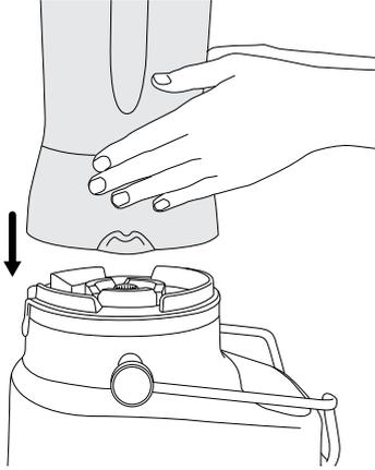
2. Raise the safety locking arm up and locate into the two grooves on either side of the blender.
