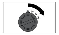
When cooking is complete, turn the temperature control dial to the OFF position, switch off at the power outlet, remove the power plug and then the connector end from the appliance inlet.
