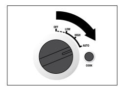
When cooking is complete, turn the temperature control dial to the OFF position, switch off at the power outlet, remove the power plug and then the connector end from the appliance inlet.
