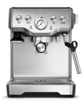
Electronic PID control improves temperature stability and a 54mm wide group head helps draw even, balanced flavours in each cup. The 1700W high power delivers fast heat up and high pressure steam for improved milk texturing.
