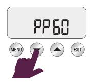
We recommend a range of between 55–65 as being optimum. Press EXIT to confirm setting and return to STANDBY mode.
