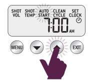
Press UP or DOWN arrow to adjust AUTO START to the desired time. (default AUTO START time set at 7:00am). Press EXIT button. Machine will beep once to confirm setting.
