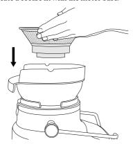
Place the juicer cover over the filter bowl surround, positioning the lower part of the feed chute over the stainless steel filter basket.
