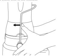
3. Add food or liquid into the blender jug ensuring not to exceed the 'MAX' mark. Place the blender lid firmly into position on the top of the blender jug. Insert the clear, inner measuring lid into the blender lid and turn clockwise to lock into position. The jug features a Breville® Assist™ Lid. This allows the lid to fit tightly onto the blender jug, avoiding displacement during operation.
