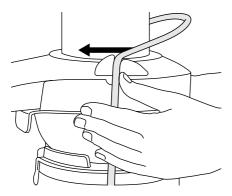
Slide the food pusher down the food chute by aligning the groove in the food pusher, with the small protrusion on the inside of the top of the feed tube.
