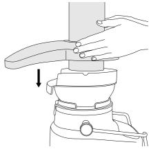
Raise the safety locking arm up and locate into the two grooves on either side of the juicer cover.
