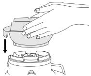
2. Align the arrows at the base of the stainless-steel filter basket with the arrows on the motor drive coupling and push down until it clicks into place to create a secure fit with the motor base.
