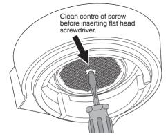
5. Once loosened, carefully remove and retain the screw and the stainless steel shower screen. Make note of the side of the shower screen that is downwards. This will make re-assembly easier. Wash the shower screen in warm soapy water, then dry thoroughly. Remove the silicone seal with your fingers or a pair of long-nose pliers. Insert the new seal, flat side first, so the ribbed side is facing you.
