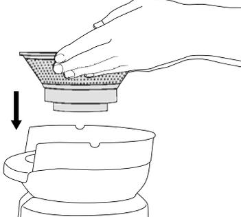
4. Place the juicer cover over the filter bowl surround, positioning the lower part of the feed chute over the stainless steel filter basket.
