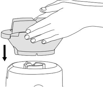
3. Align the arrows at the base of the stainless steel filter basket with the arrows on the motor drive coupling and push down until it clicks into place to create a secure fit with the motor base.
