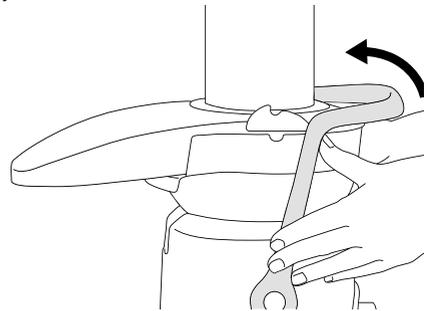
6. The safety locking arm should now be in a vertical position and locked into place on top of the juicer cover.
