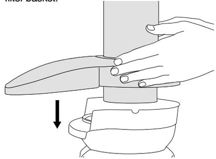
5. Raise the safety locking arm up and locate it into the two grooves on either side of the juicer cover.
